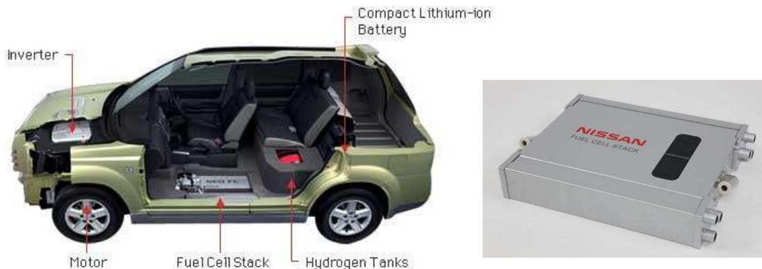
*Figura 57. Nissan X-TRAIL FCV e Nissan fuel cells stack*
