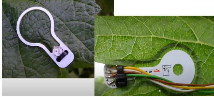
Figure 4: FYLLO CLIP sensor mounted on a grapevine leaf (FruitCREWS, 2023)
