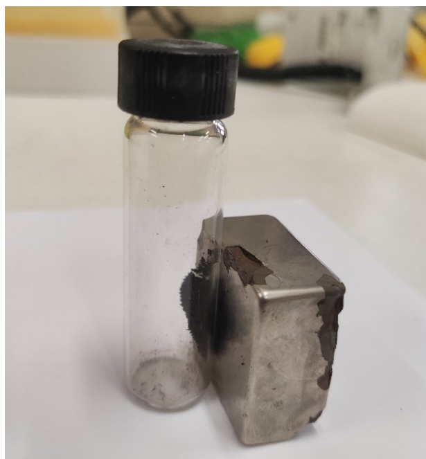
Figure 8.4: Magnetite nanoparticles powder, attracted by a permanent magnet.
