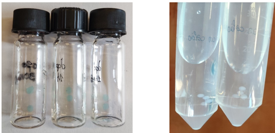
Figure 9.13: Beads removed from the solution after respectively 30 min, 1 h and 1 h and 30 min (on the left). Regenerated beads in calcium solution (on the right).
