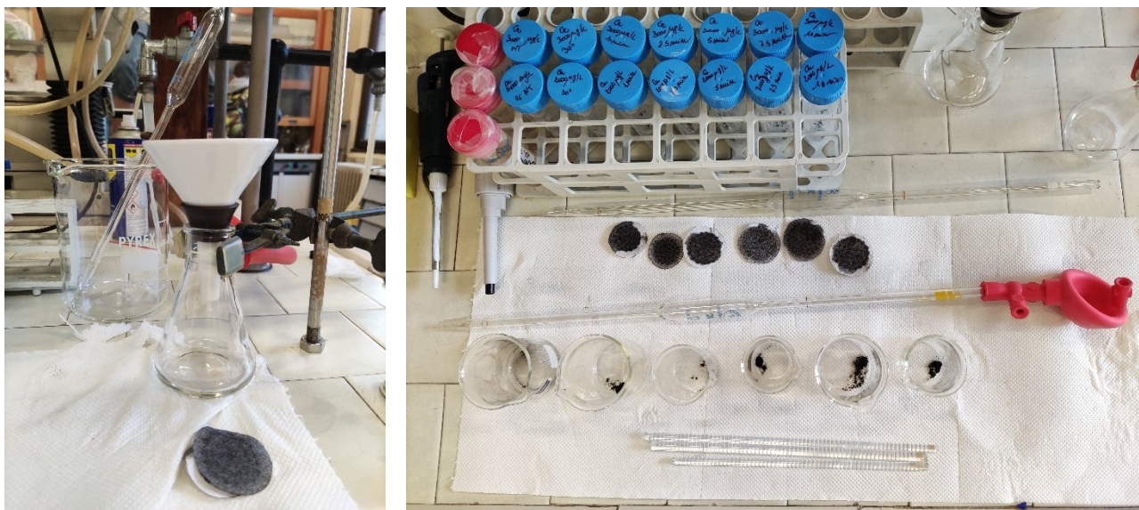
Figure 8.13: Filtration apparatus (on the left). Test apparatus for adsorption tests with nanoparticles (on the right).
