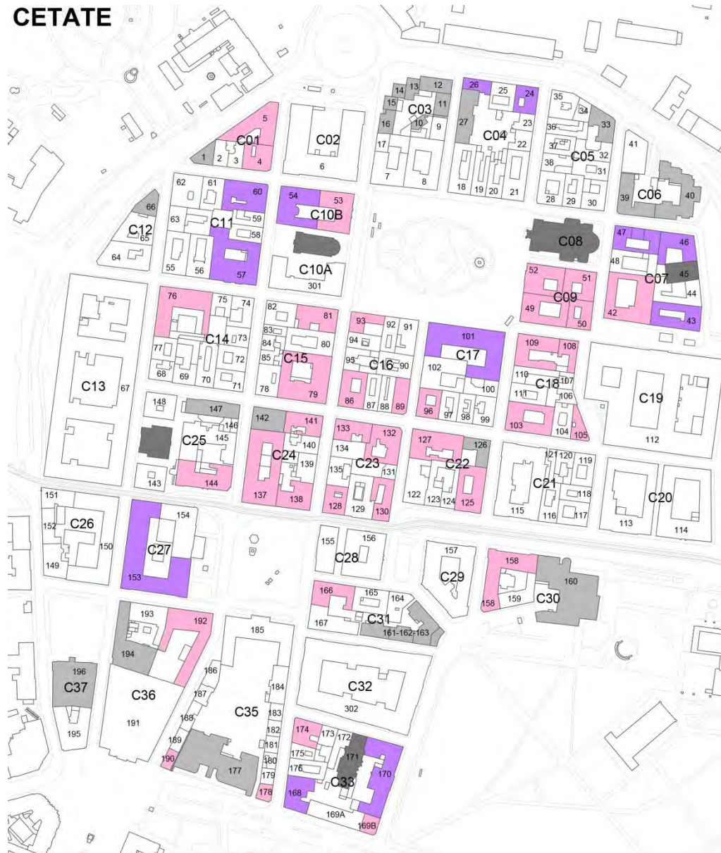
Fig. 6.6.4: Vulnerability assessment of PL1 - in-plane mechanism
