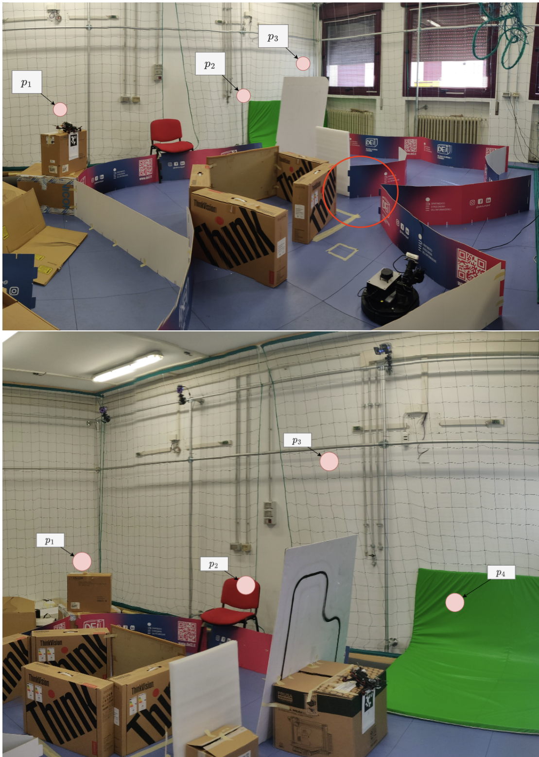
Figure 5.19: Snapshots of real world experiment #2. In red there are reported the positions in which the quadcopter will stand during the second phase of the experiment. The circle in red on the first picture instead represents the dynamic obstacle
