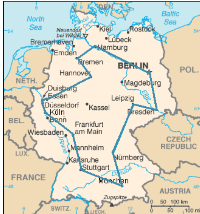
Fig. 1. 2: An optimal TSP tour through Germany's 15 largest cities. It is the shortest among 43589145600 ( 14!/2 ) possible tours visiting each city exactly once, Central Intelligence Agency (2007)
