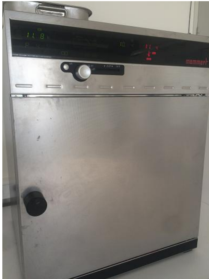
FIGURE 25 OVEN SET AT 10 DEGREES FOR THE STORAGE OF THE SAMPLES
