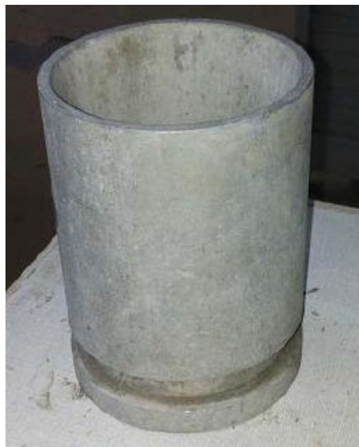
FIGURE 16 MINI- CONE ABRAMS
