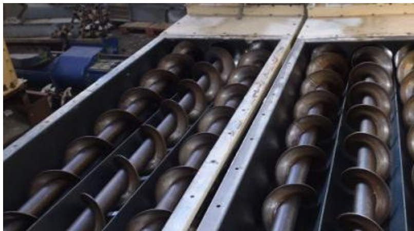
FIGURE 2 BAUER TRIPLE AUGER
