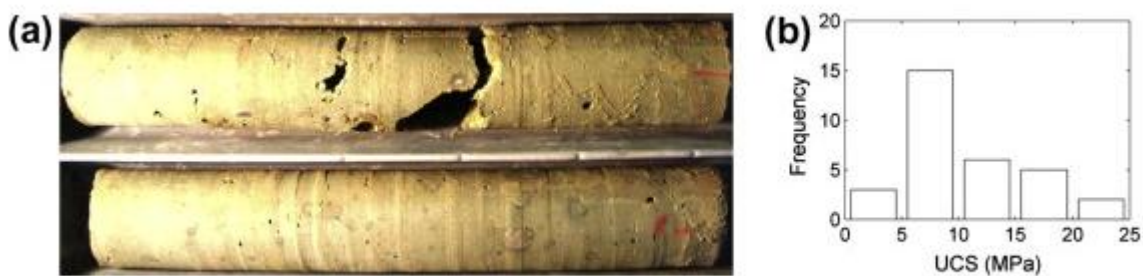
FIGURE 11 TWO CORES WITH A LENGTH OF ABOUT 550 MM FROM THE SAME SOIL-MIX PANEL. THE SOIL IN THE INCLUSIONS WAS WASHED OUT DURING CORING. HISTOGRAM OF 31 UCS VALUES OF SOIL-MIX SAMPLES FROM A CONSTRUCTION SITE IN BELGIUM (LOAM)
