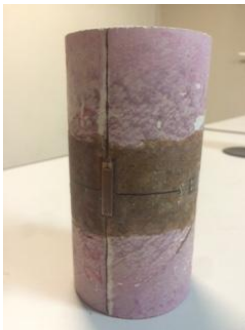
FIGURE 41 SAMPLE 7x14 WITH VERTICAL AND HORIZONTAL GAUGES GLUED
