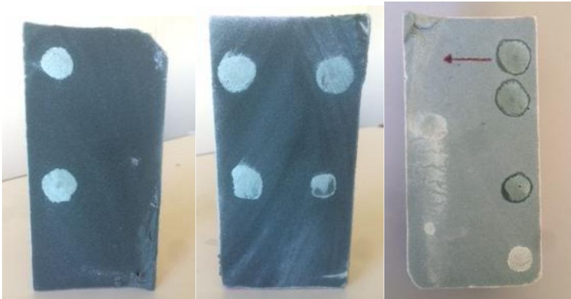
FIGURE 32 CUT OF SAMPLE WITH 1, 2, 3 INCLUSIONS PER LAYERS
