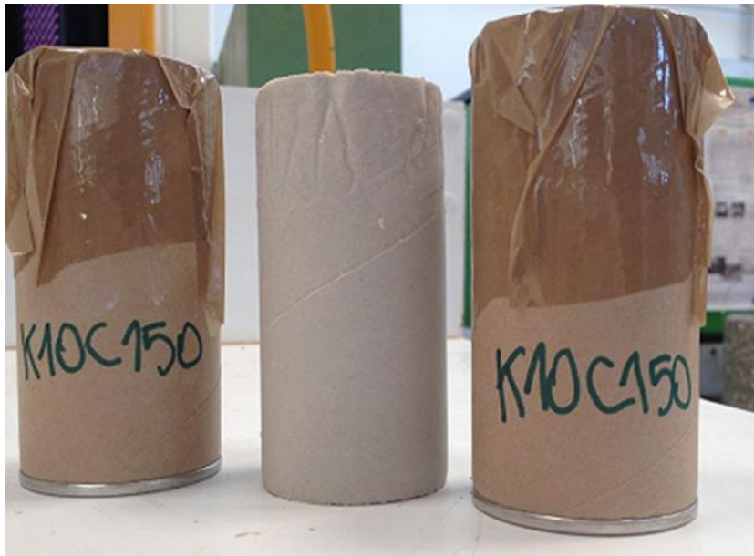
Figure 23 Moulds 5x10 and sample after 7 days of storage
