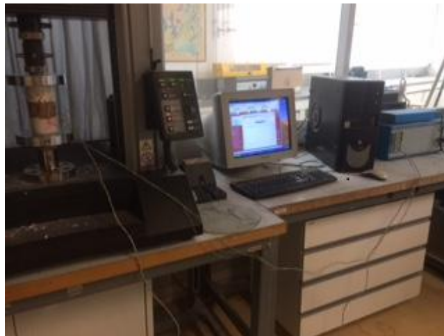
FIGURE 39 INSTRON USED FOR THE CYCLIC TEST
