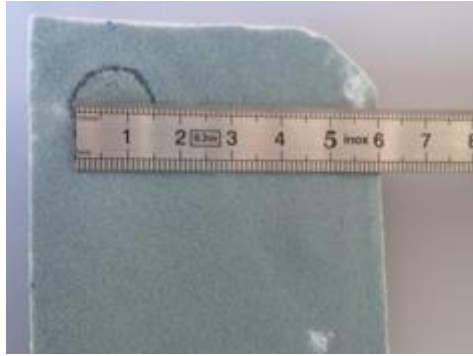
FIGURE 35 DIAMETER OF A CLAY INCLUSION 1,5 CM
