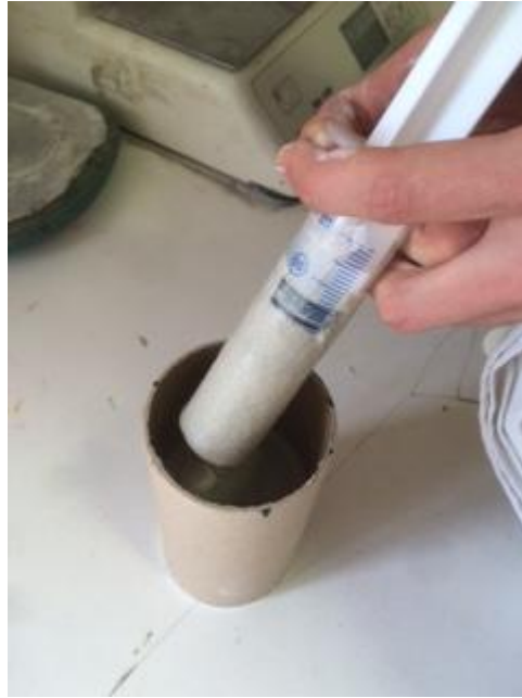
FIGURE 26 MOLD 7x14 FILLED UP OF FRESH MATERIAL WITH A SYRINGE
