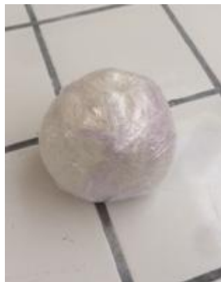
FIGURE 34 MIX OF CLAY AND WATER USED TO MAKE THE INCLUSIONS
