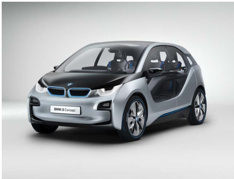
Figure 1.7: BMW i3 electric car. The frame and the skin are both made with composite materials. http://articles.sae.org/11618/
