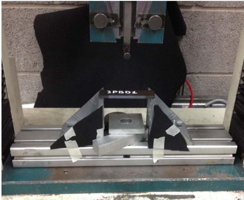
Figure 5.10: Experimental configuration for the three point bending test.
