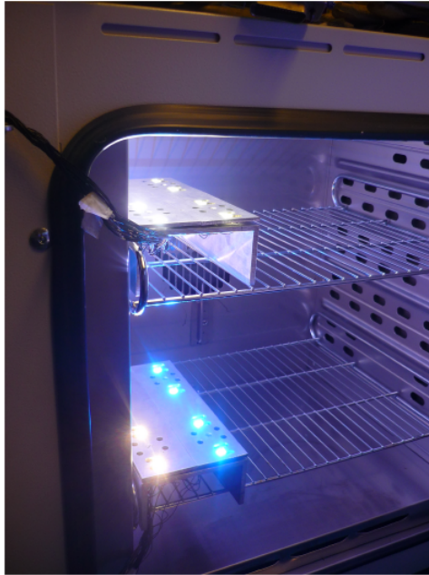
Figure 4.2: Two eight LED aluminium blocks under stress in oven
