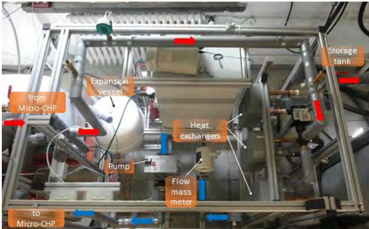
Fig.3.1.2 - Heat exchange module's scheme
