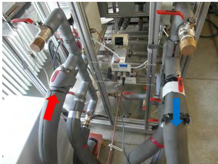
Fig.3.1.4 - CHP's side of the heat exchanger module
