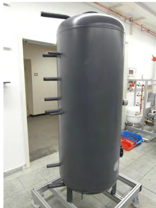
Fig.3.1.9 - Storage tank without external
