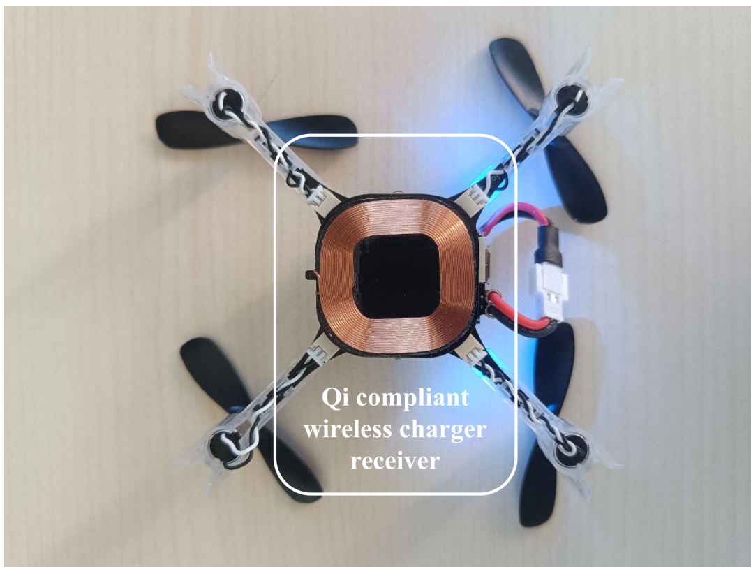
Figure 2.5: Wireless power transfer using Qi
