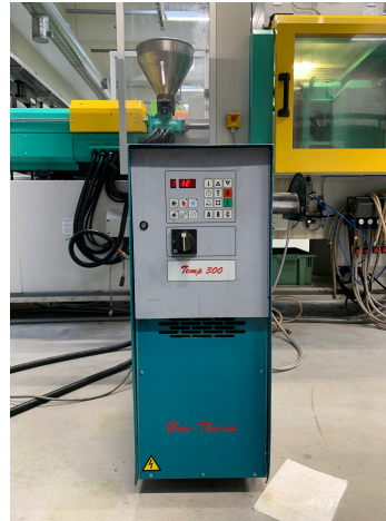
(b) Mold Temperature controller
