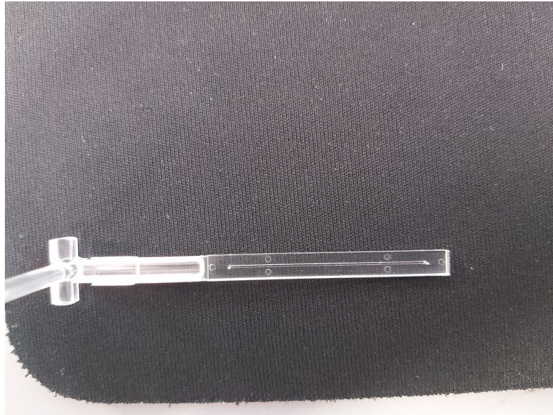
Figure 4.2: Picture of a molded part. The micro-channel can be seen as well as 6 ejector pins marks and the two holes.
