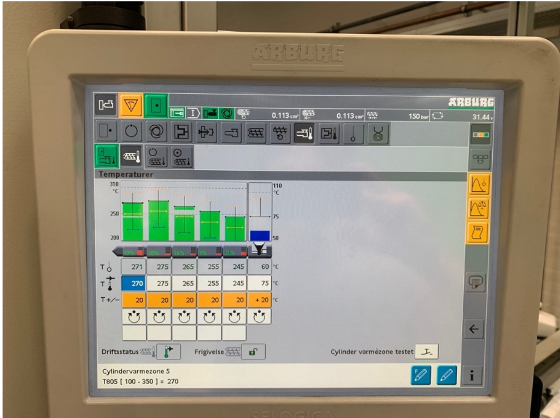
Figure 4.5: Boundary conditions. The melt temperature profile through the barrel. Note the temperature near the hopper is lower to avoid the pellets stick in the barrel.
