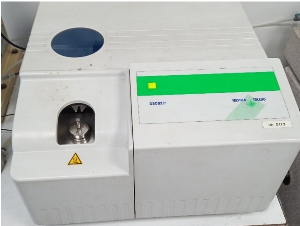
Figure 4.1: Mettler-Toledo DSC 821 utilized for the whey protein isolate denaturation analysis in the laboratory of the IQS.
