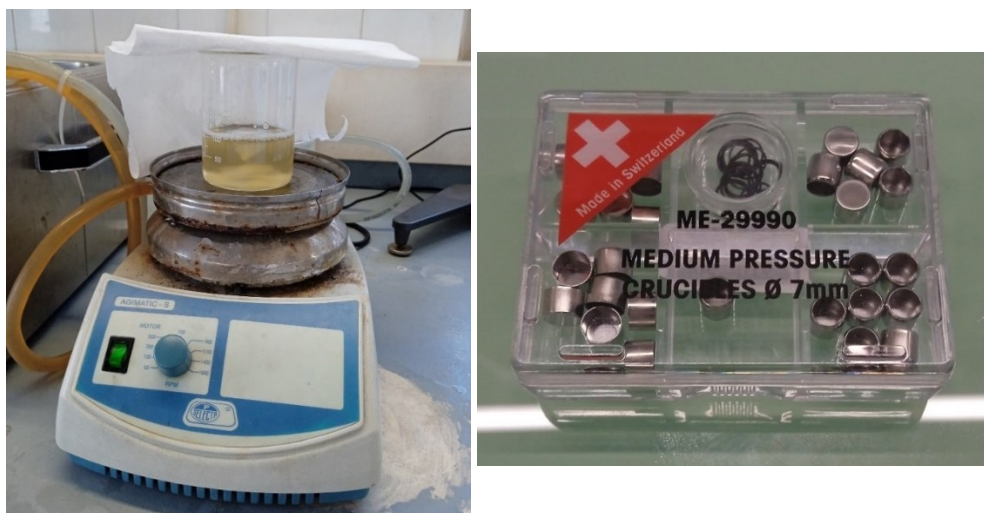
Figure 4.2: WPI solution preparation through a magnetic mixer (left) and medium pressure crucibles pans utilized for the WPI denaturation analysis under DSC (right). The diameters of the crucibles were about 7 mm.
