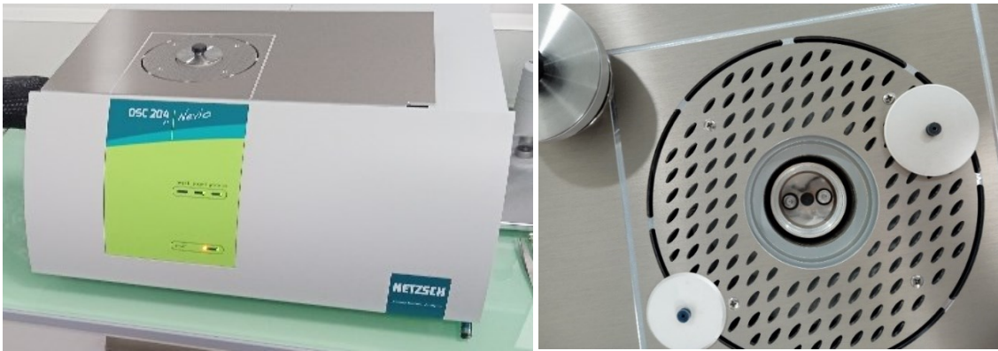
Figure 4.6: Netzsch DSC 204 utilized for the sol-gel transition analysis in the laboratory of the IQS. On the left is shown the machine from the outside, while on the right it can be observed the DSC cell in which the pans and the reference are put.
