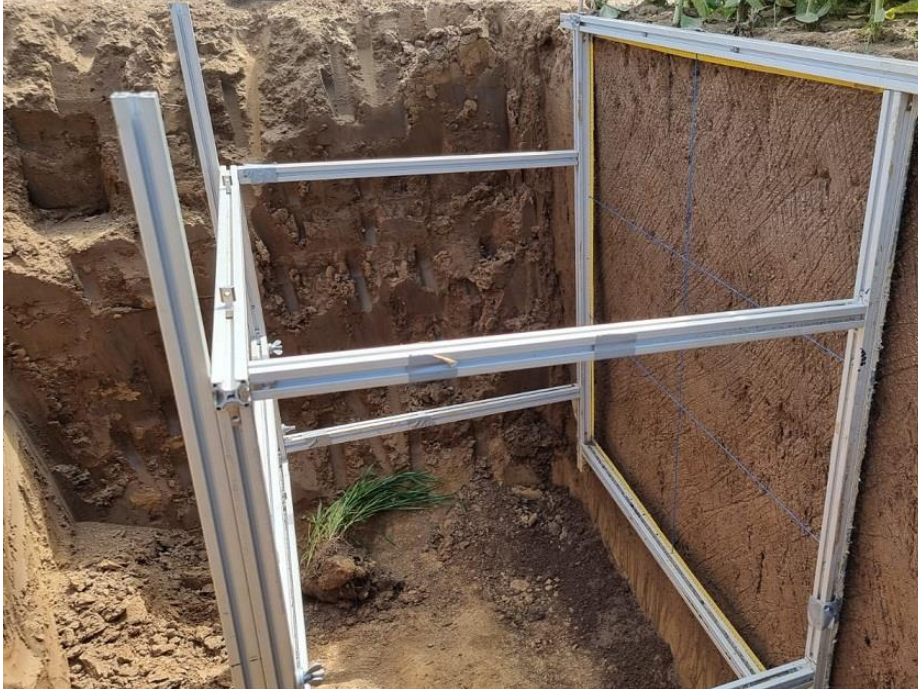
Figure 5: Measuring RLD ( \text{cm}/\text{cm}^2 ) by using 100 x 100 cm frame (partitioned into two vertical (50 cm each) and three horizontal portions (35 cm, 30 cm and 35 cm) with profile wall method. Source (by Zia Ullah and Arslan) (Date: 2nd June 2022) (Location: Campus Klein-Altendorf)
