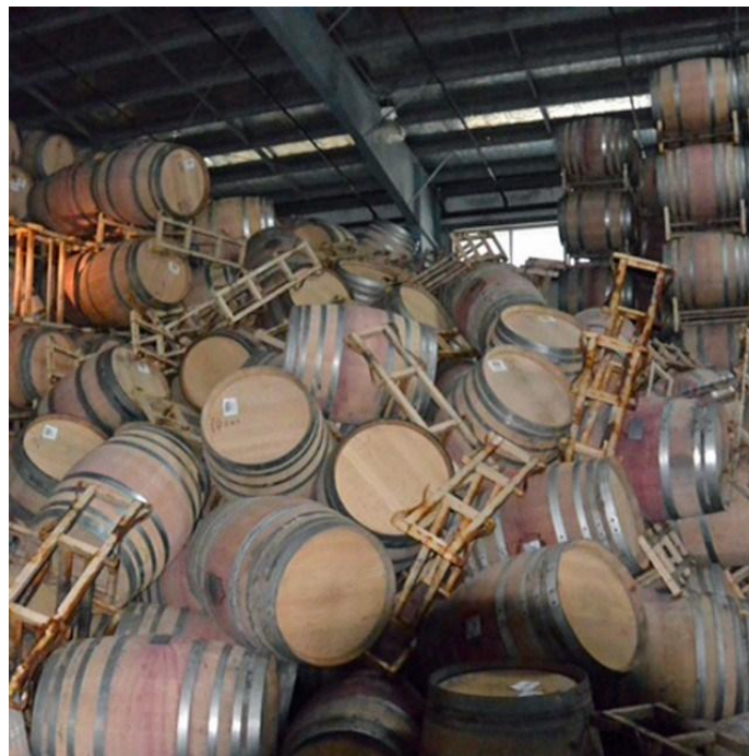
Fig 1.4: Support barrels failure in a Napa winery.
