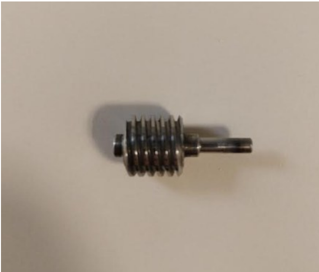
Figure 47: view of worm gear
