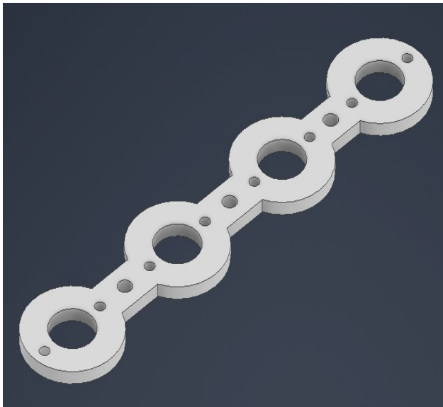
Figure 18: frame for flanging the 4 gear motors
