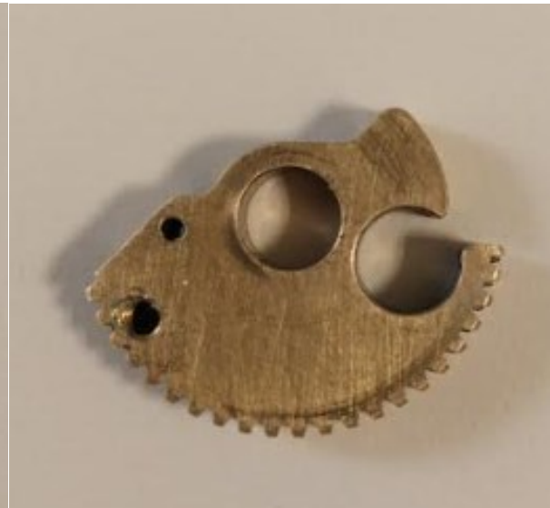
Figure 48: view of the gear frame
