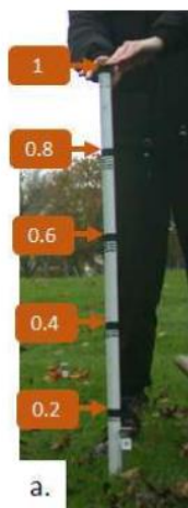
Figure 1.3 Calibration pole, from: Field protocol for camera trap surveys with camera calibration for measuring animal positions for unmarked density estimation (Rowcliffe, 2022).
