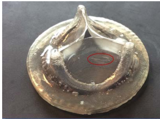
Figure 8.12: SESP22 Broken Valve.
