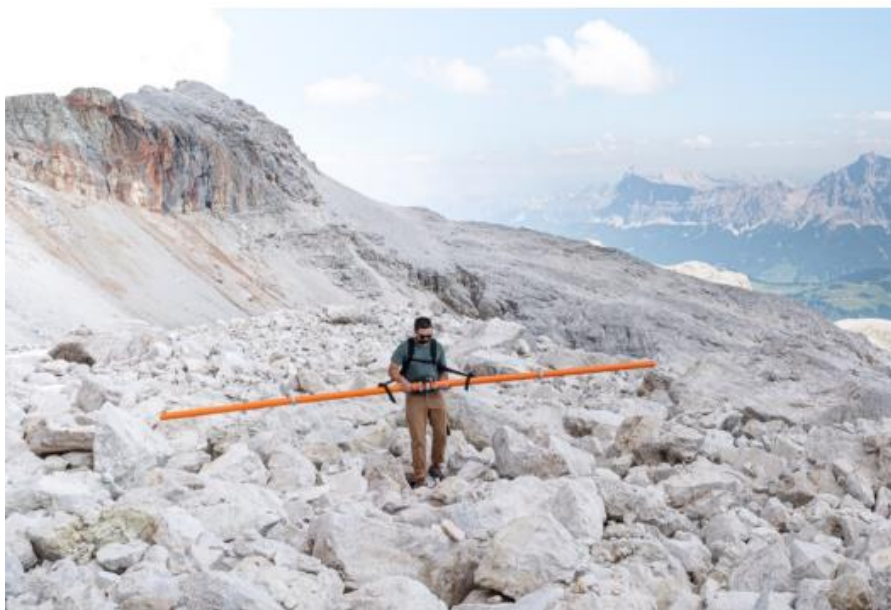
Figure 37: Electromagnetic Measurements Using the CMD-Explorer at the Piz Boé Rock Glacier Site. Photo by Boaga, 2020
