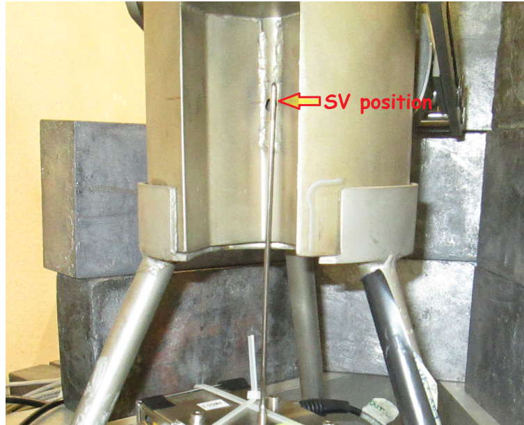
Figure 5.1: Picture of the AMiCo 6 detector placed in the gamma irradiator housing the radioactive source.
