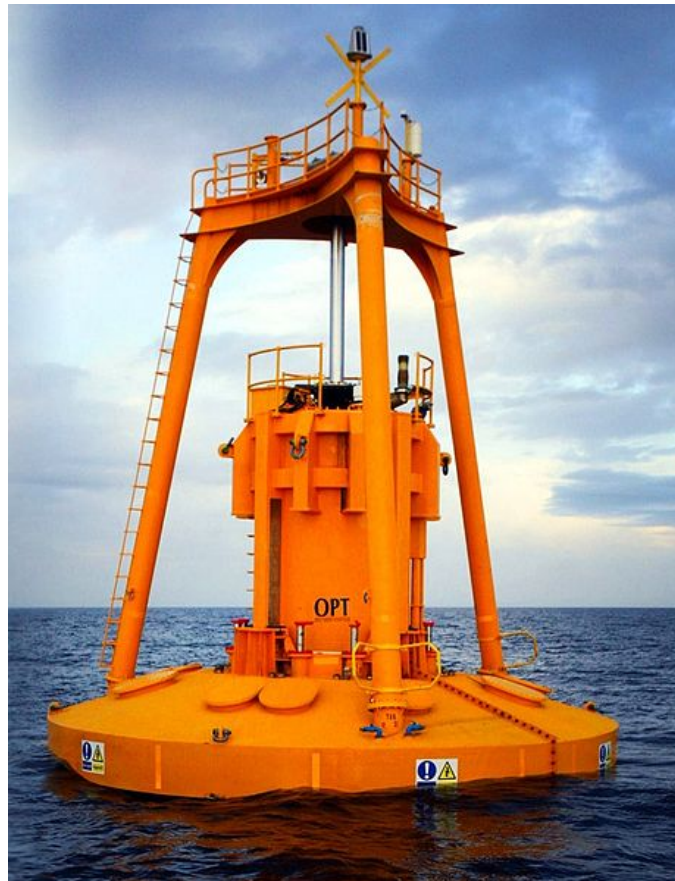
Figure 1.6: PowerBuoy with peak-rated power output of 150 kW.
