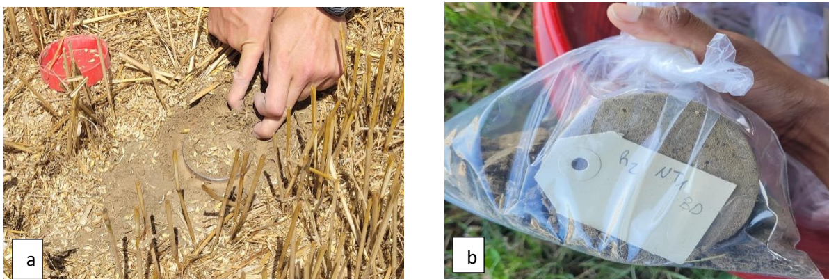
Figure 10: a. Samples (Bulk density) are collected from the top 5cm of soil b. Soil sample
