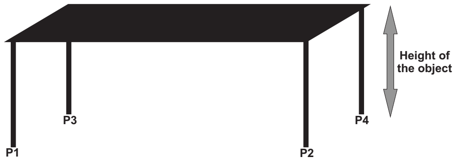
Figure 8.3: The mapping of a desk: the four feet form a rectangular base, that includes all edges of the desk. The parallelepiped that include the desk is defined multiplying the base with the desk height.
