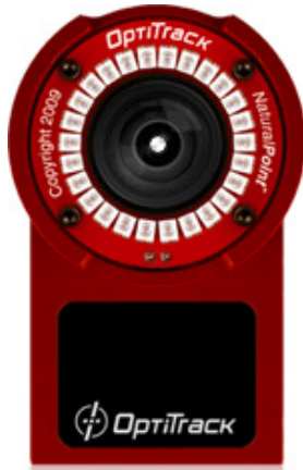
(a) An OptiTrack camera, used by the MoCap system installed at IPEM. IR LEDs surround a infrared sensor (like a camera, in the middle)
