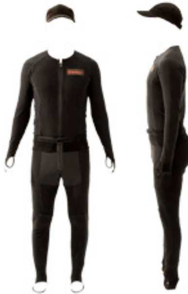
(d) Motion Capture suit, markers can be attached to any of the velcro-friendly surfaces.
