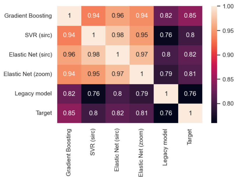
Figure 5.2: Comparison of the prediction of the different models on the test set via Pearson correlation
