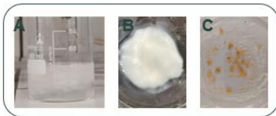
Fig. 39: Dissolution steps of the cotton-based fibre in NaOH/glycerin solution.
