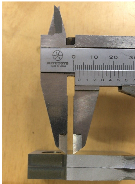
Figure 21: Crack size symmetry validation for an LIMC specimen.
