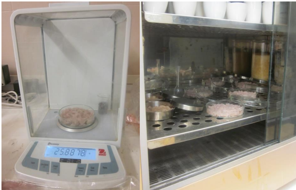
Figure 11. On the left an example of the weighted sample and on the right samples put in the drying oven
