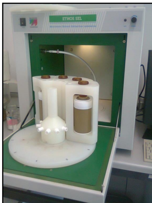
Figure 25. Microwave oven Milestone Ethos Sel model with representation of the loading of the samples
