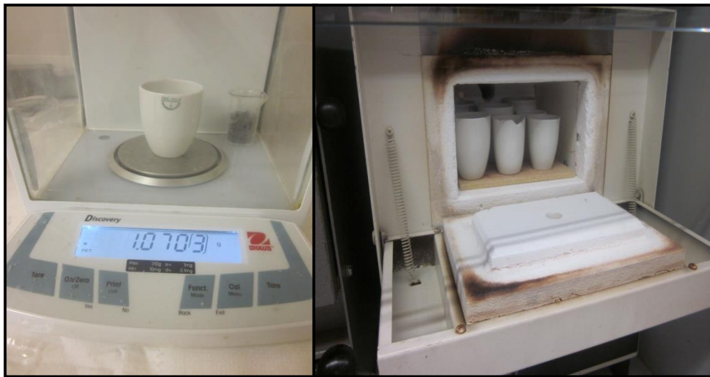
Figure 18. On the left: weighing the fresh sample; on the right: samples placed into the Program Controller S27 muffle furnace
