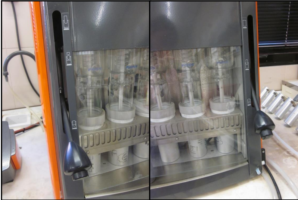
Figure 17. Some details of Soxhlet extractor: on the left the first two phases, on the right phases 3 and 4
