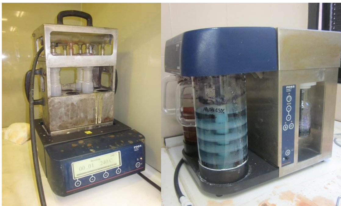
Figure 12. On the left a Kjeldahl digester working; on the right a scrubber
