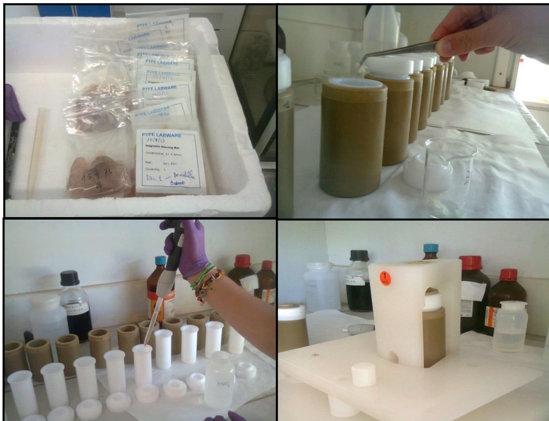
Figure 24. Series of pictures representing the preparation procedure of the samples to place in the Microwave solvent Extraction lab station
