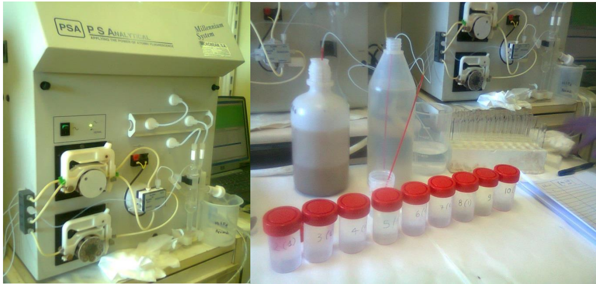
Figure 27. Atomic fluorescence spectrophotometer PSA Analytical Millennium system and some samples subjected to analysis
