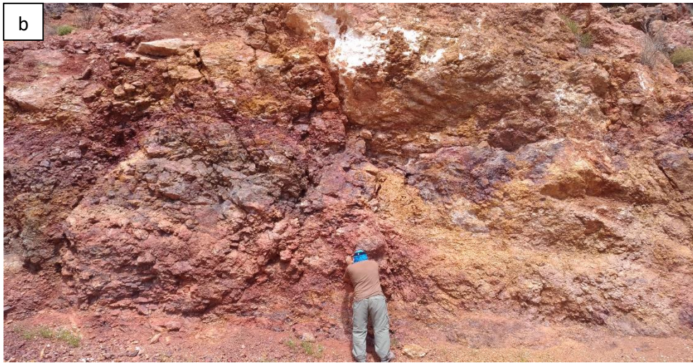
Figure 5.34_a) View of the limonitic gossan (red ellipse) from wpt.15. b) Limonitic gossan, formed by a solid gel of hematite, goethite and jarosite wtp.18.
