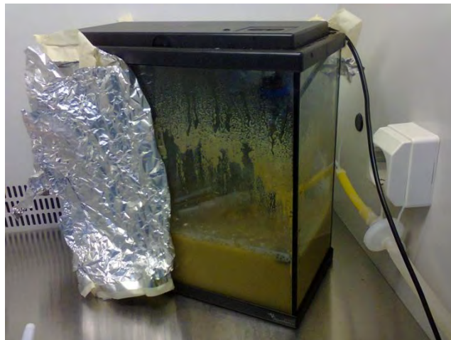
Figure 2.2. Chlorella protothecoides grown in aquarium with fed-batch strategy and pH control
