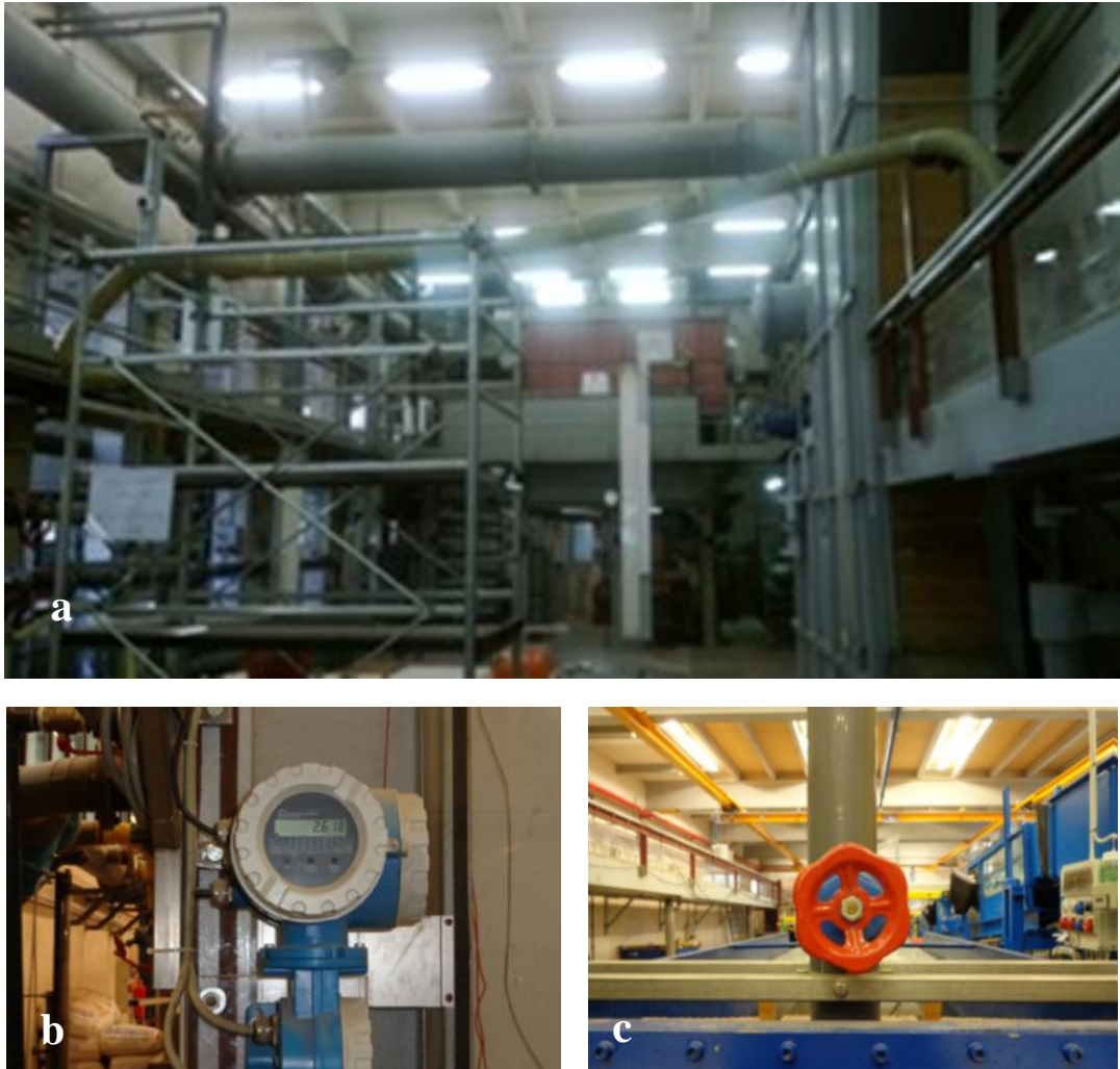
Fig 2.4: The flow regulation. (a) The head tank, (b) the flow meter and (c) the crank.
