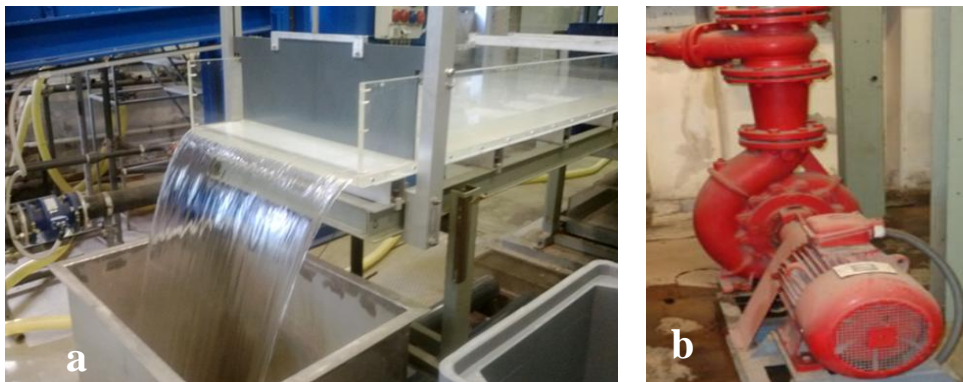
Fig 2.3: The flume's components. (a) The gate and (b) the centrifugal pump.
