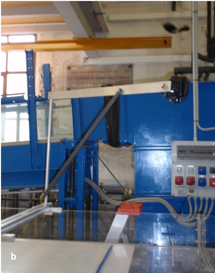
Fig 2.5: Flume's accessories to carry on the tests: (a) wall of brick, (b) camera's support.
