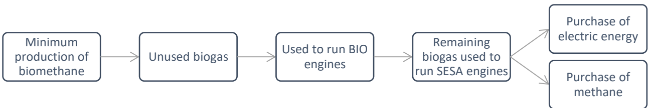
Figure 18: minimum biomethane production, remaining biogas used to run firstly BIO engines and, if some biogas is still available, to run SESA engines.
