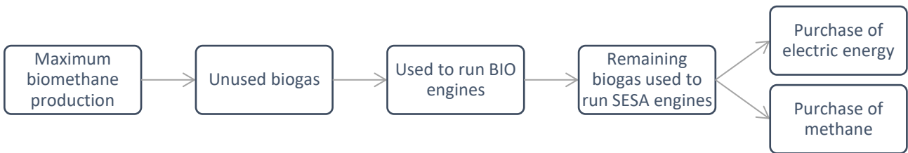
Figure 21: maximum biomethane production, remaining biogas used to run firstly BIO engines and, if some biogas is still available, to run SESA engines.
