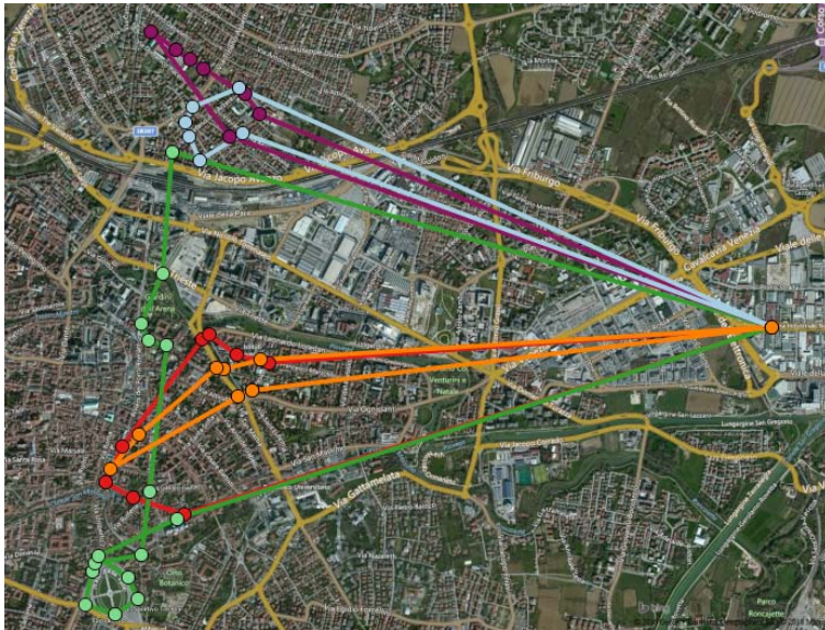
Figure 4.47: Three-phase Algorithm routes planning after 100 iterations ( N = 100 at level 1) implemented on QGIS platform on Bing map.
