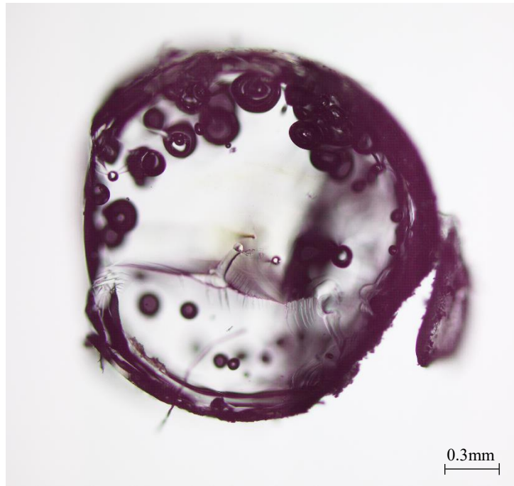
Figure 3.20: MD21 Filaments extruded at 185°C, cross sectional image.
