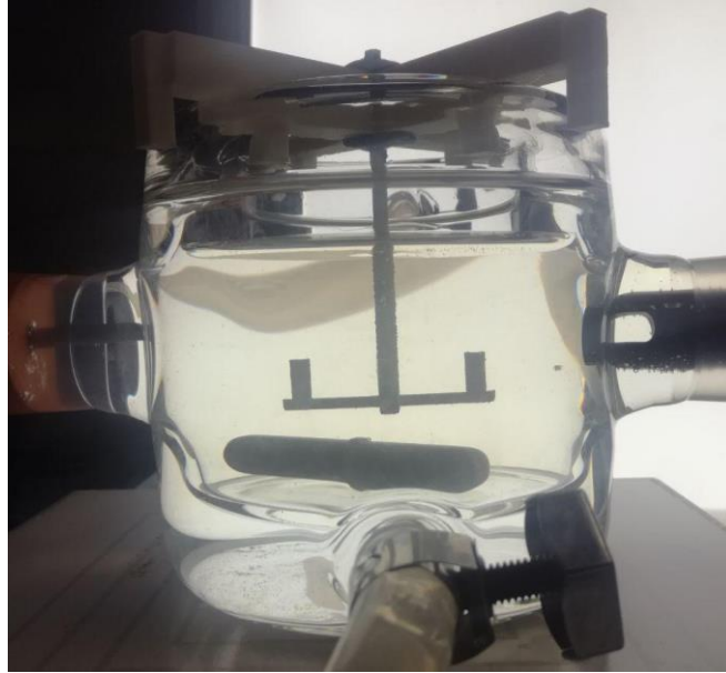
Figure 2.18: Dissolution test set-up.
