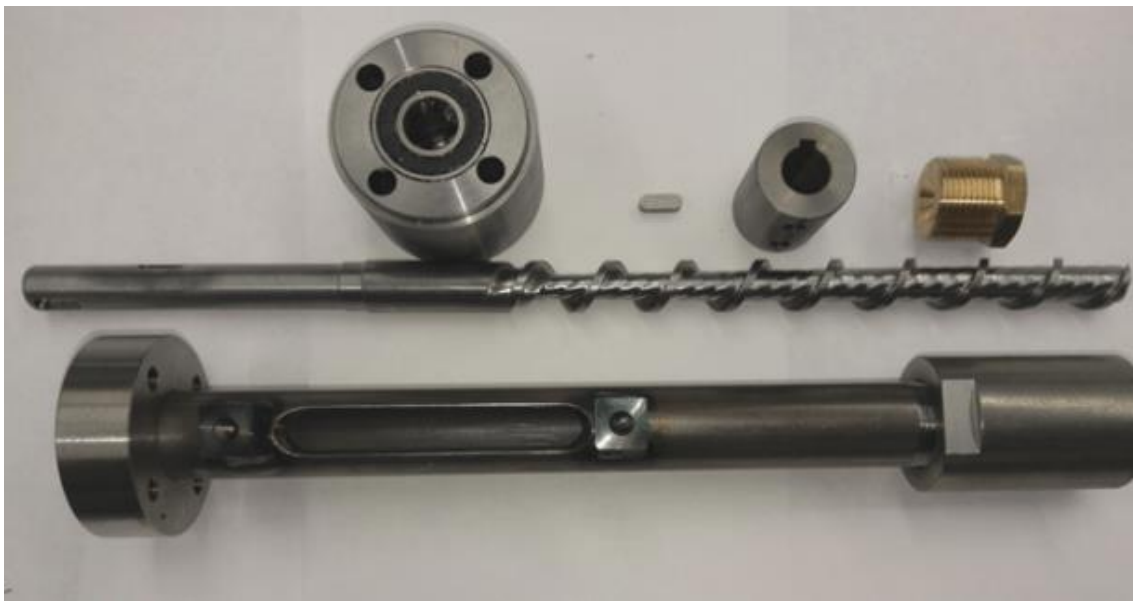
Figure 3.12: Details of the barrel and of the screw of the noztek extruder.
