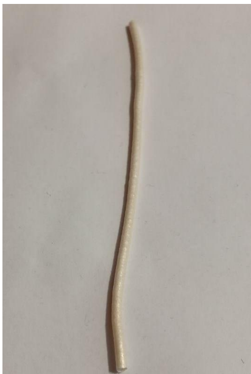
Figure 3.15: MD19 Filament extruded at 140°C, powder moisture content equal to 8.5%.
