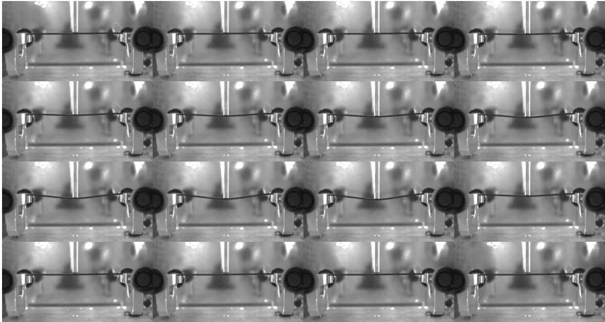
Figure 3.26 Pseudo 3 points bending test on ABS filaments. Time between 2 consecutive frames= 0.35 s.
