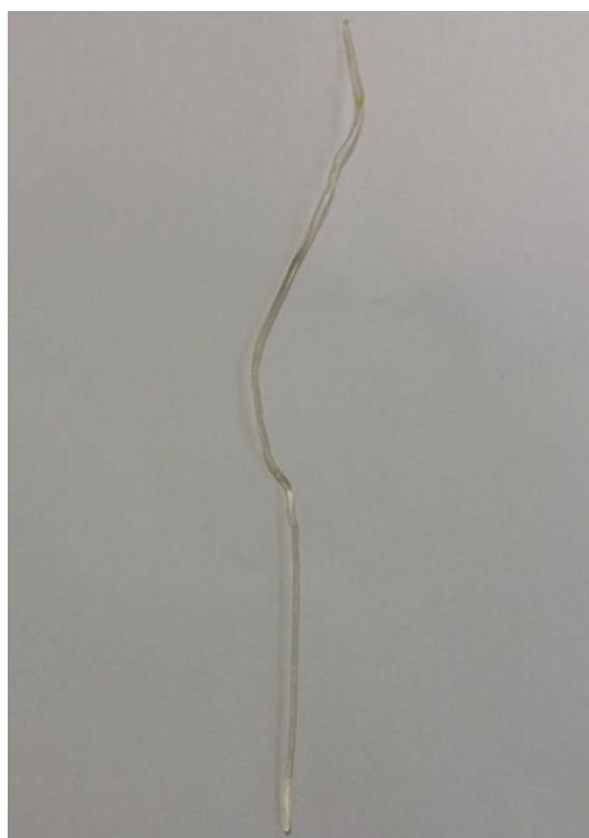
Figure 3.16: MD19 Filament extruded at 140°C, powder moisture content equal to 6.5%.
