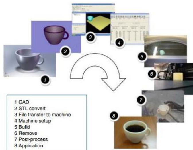
Figure 1.4: Generic Additive Manufacturing process [11]
