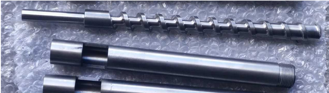
Figure 3.17: Screw and barrel of the Filafab extruder.
