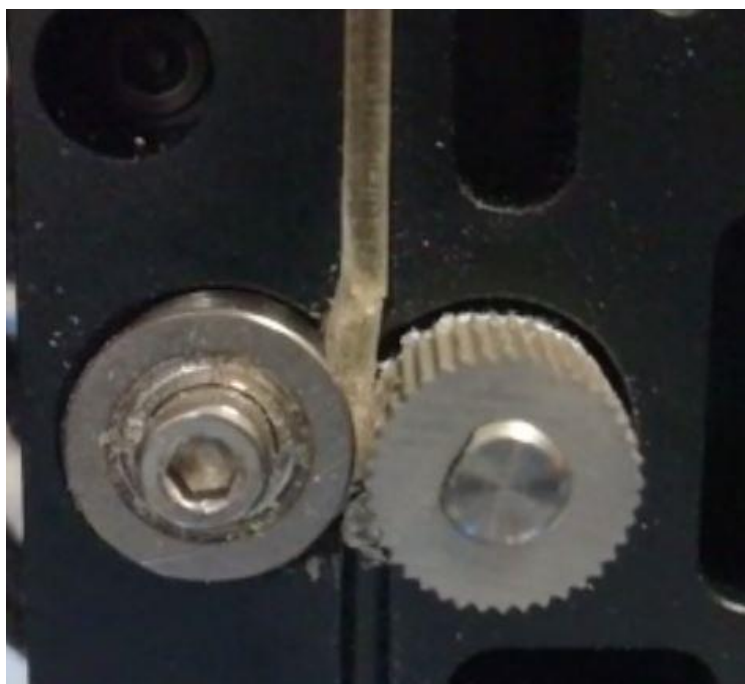
Figure 3.32: Detail of the pulling system of the Raise 3D printer loaded with MD21 filaments stored at 40% RH. The filament stored at 70% RH for one day has a higher diameter and cannot pass through the pulling system. Hence, no more tests are performed with the available MD filaments. Filaments with a smaller diameter and higher resistance are required.
