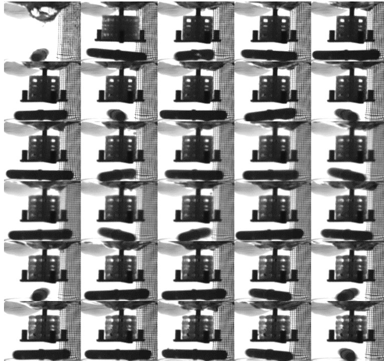
Figure 4.18: Montage of the dissolution test of geometry G1. Time between 2 consecutive frames= 1.5 min.
