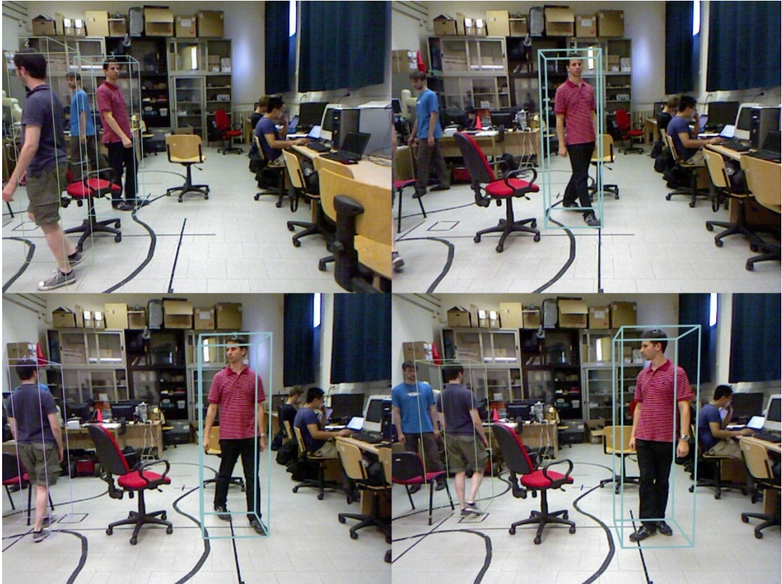
Figure 7.8: An example of track recovery. Track #2 becomes #4 after the full occlusion, but, in a few frames, it returns to its original ID.
