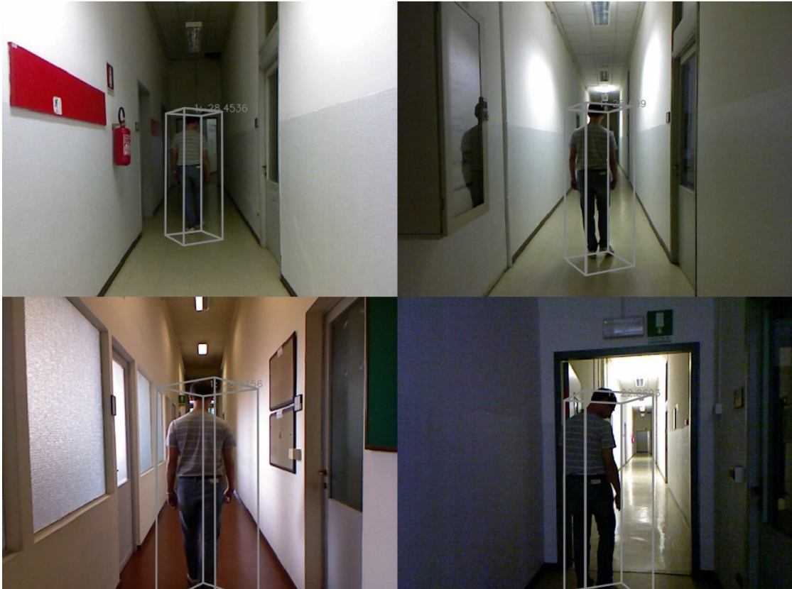
Figure 7.12: People following test: examples of tracked frames while a person is robustly followed along a narrow corridor with many lighting changes.
