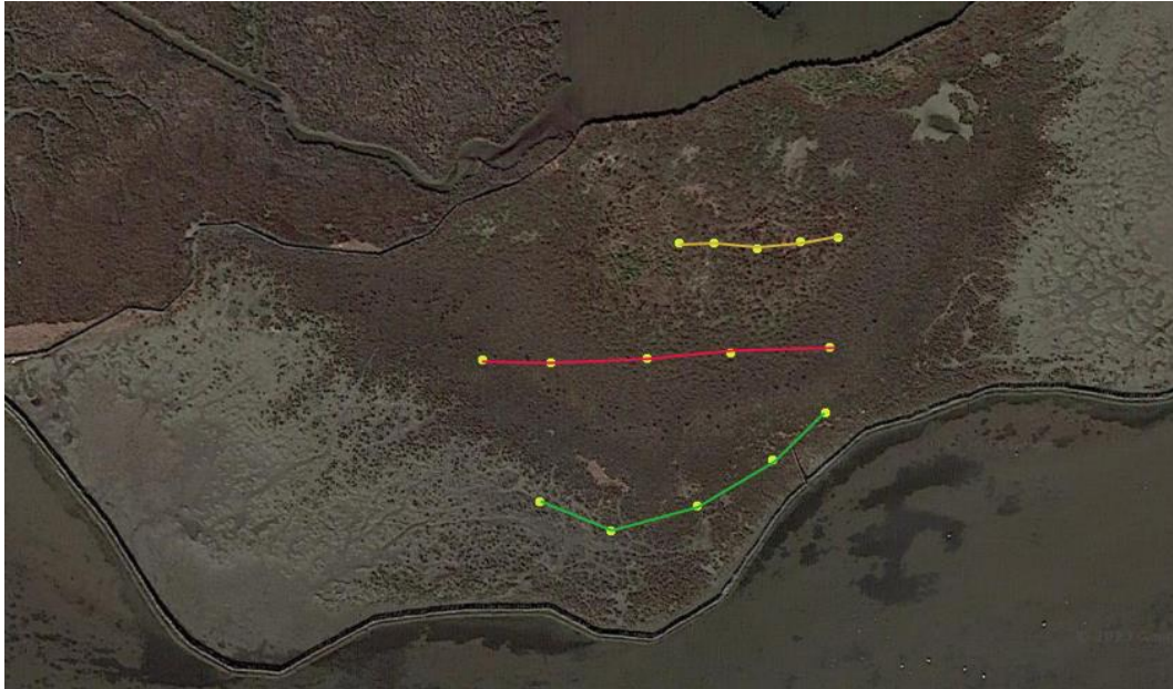
Fig. 29, Image created with QGIS software. Transects were made using salt marsh B&A data acquired by the GNSS altitude instrument (GeoMax zenith GNSS), and the map was created afterwards. Low altitude areas are shown in green, medium altitude areas in red, and high altitude areas in yellow.
