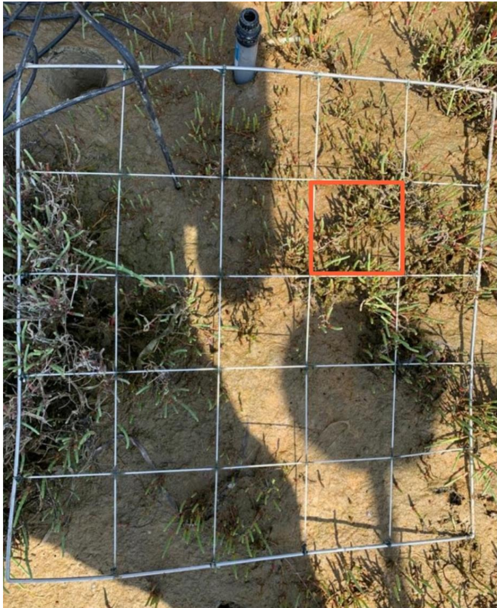
Fig. 30, Photo taken on the field, showing the quadrat used and the redox potential survey tool EcoTech (on top). One of the square units is highlighted in orange, constituting 4% of the total.
