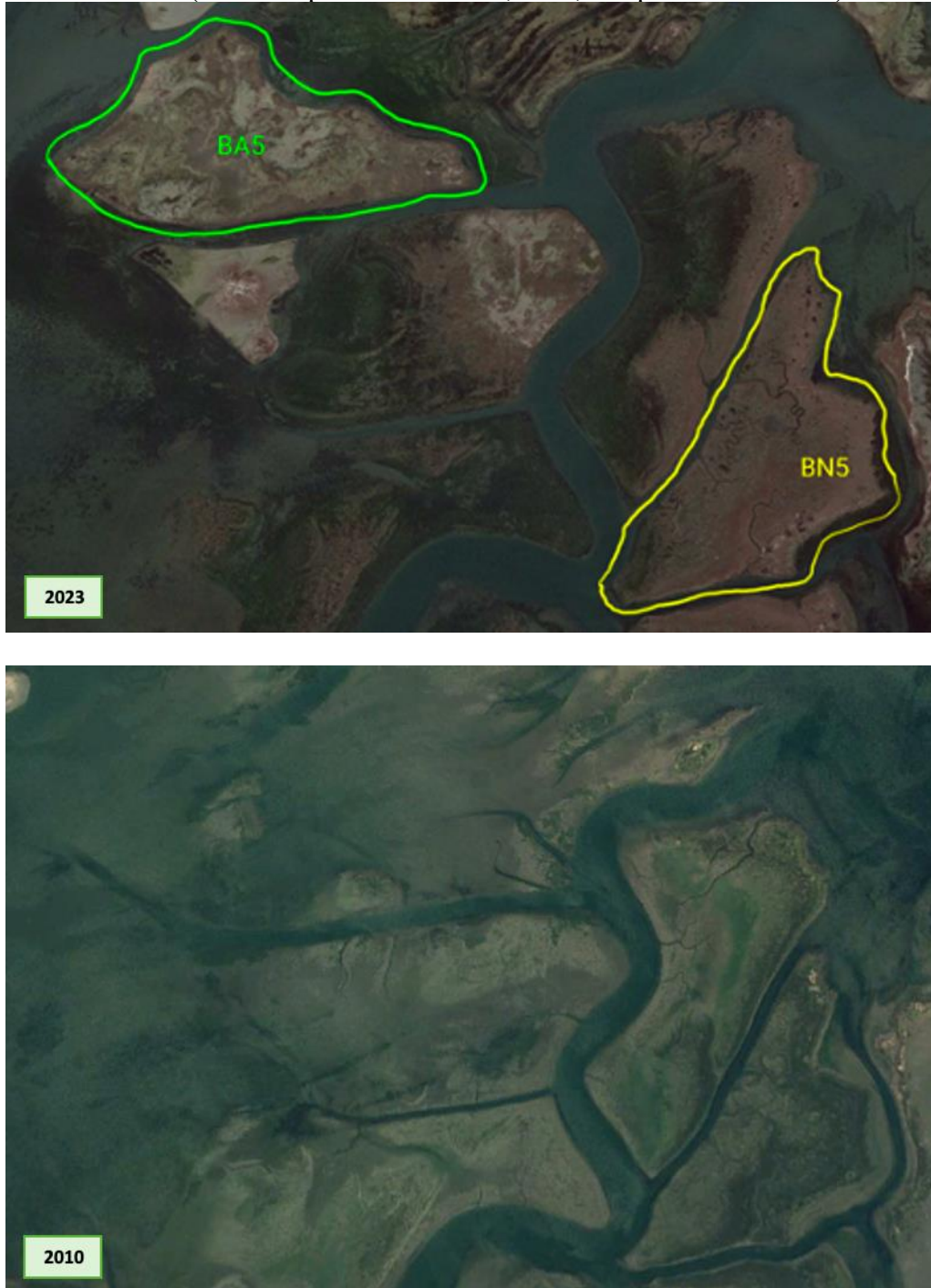
Fig. 21 Image obtained from Google Earth, using "historical imagery" instrument. Each salt marsh has been tagged with the letter B ("Barena") and the adjective N (natural) or A (artificial). The comparison between before the construction of the artificial salt marsh (BA5) and after is visible; 2023 vs 2010.
