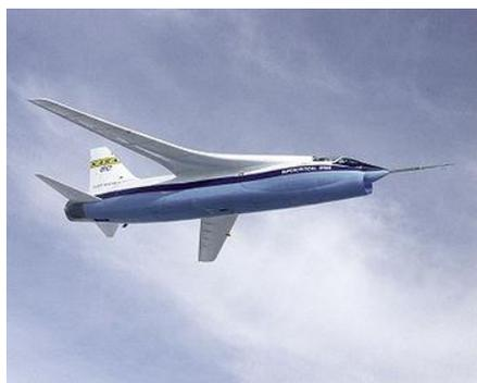
**Figura 4.1:** NASA TF-8A, testbed ala supercritica ([www.nasa.gov](http://www.nasa.gov)).
