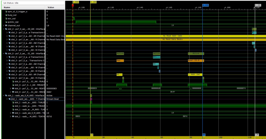
Figure 3.11: AXI-stream compared with AXI-Lite, showing that the data is streamed 12 T_{CLK} after the EOC, against the \approx 90 clock cycles required by the PS to fetch the data, and the 125 required to execute the algorithm
