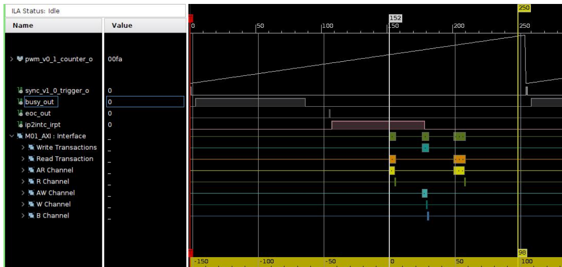
Figure 3.10: XADC interrupt handler showing that the EOC interrupt is served and cleared approximately after 50 T_{CLK} cycles, and the ADC value read after other 50 clock cycles
