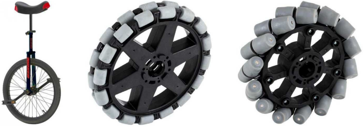
Figure 2.1: Different examples of wheels: (left) standard wheel, (middle) omniwheel, (right) mecanum wheel.
