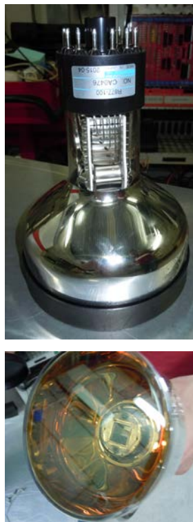
Figura 9. PMT HAMAMATSU R877-100
