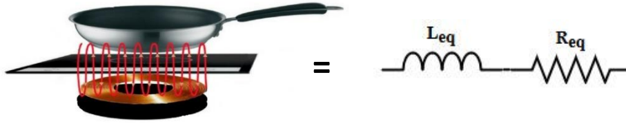
Figure 3.2: Lumped parameters model of the inductor and load system
