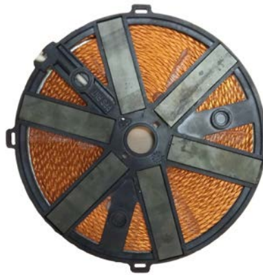
Figure 6.1: View of the bottom part of the inductor where the ferrite bars are placed
