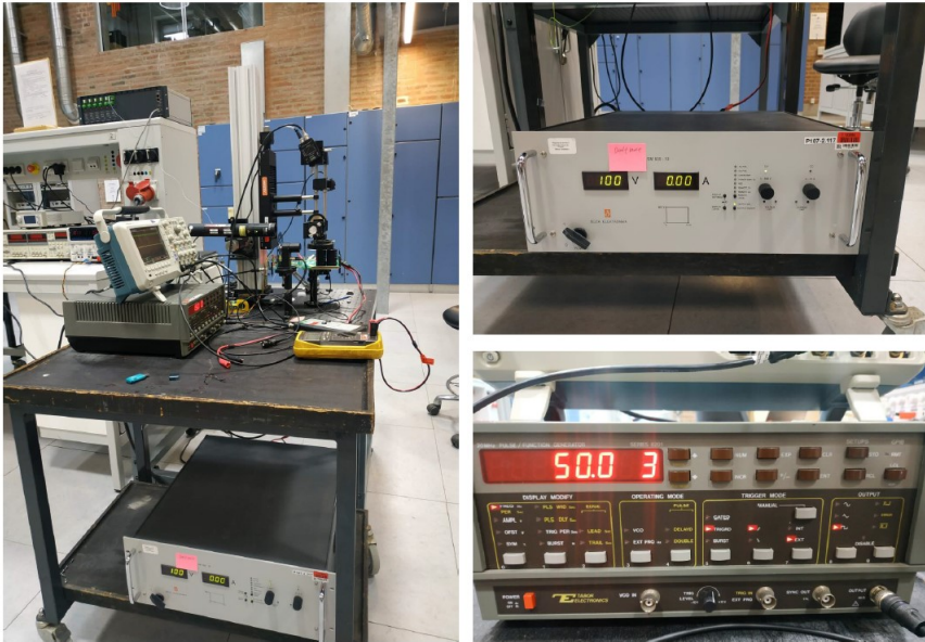
Figure 5.23: Laboratory setup for conducting short-circuit measurements
