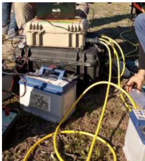
Figure A.2. Mangusta geo-resistivity meter from AMBROGEO (from data project)
