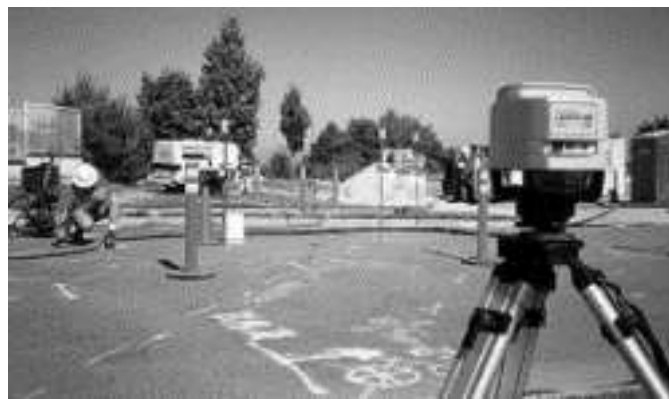
Figure 2.7. Rotating laser level for heave monitoring (ASCE, 2010)
