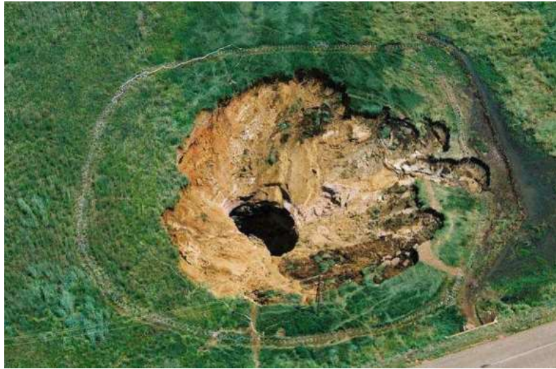
Figure 1.11. Dewatering induced sinkhole in South Africa (Council for Geoscience, 2011)
