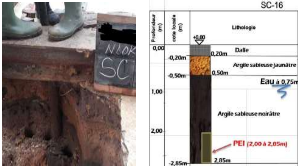
Figure 4.14. SC 16 excavated point & lithology
