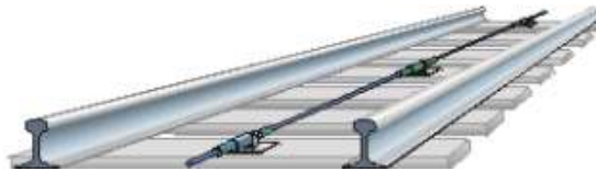
Figure 4.50. Sketch of a clinometer measuring railway settlements
