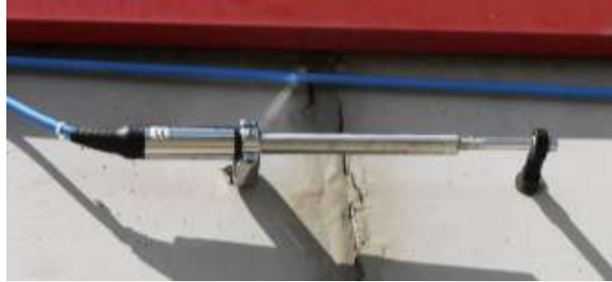
Figure 4.49. Different sizes of fissuremeters (sisgeo.com, 2021)
