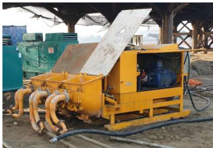
Figure 2.21. Pump for Multiple Simultaneous Compaction Grouting (Hyobum et al., 2019)
