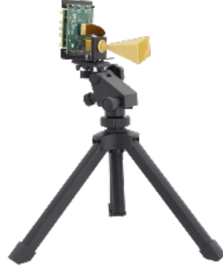
Figure 5.3: The Vubiq development system, equipped with a 60 GHz horn antenna, employed as a receiver.
