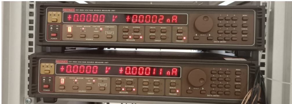
Figure 1.15: The two Keithleys 237 used for reverse current measurements as a function of reverse bias voltage
