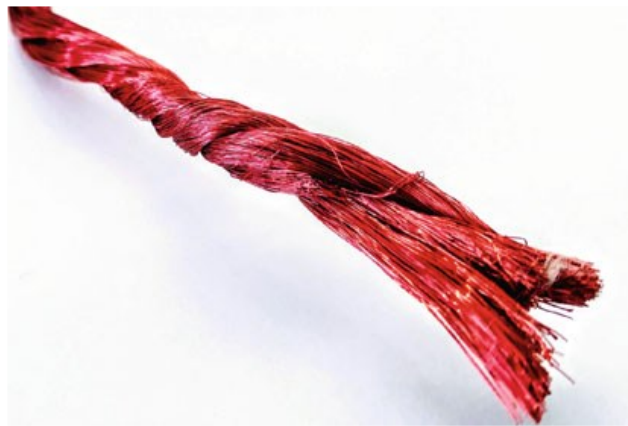
FIGURE 2.13 - SECTION OF A LITZ WIRE
