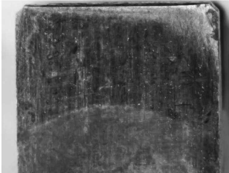
Figure 12.12: Transformation curve on the middle of the tip
