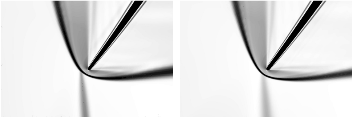
Figure 6.26: Numerical Schlieren pictures of the leading-edge for \sigma = 1.47 and \sigma = 1.60
