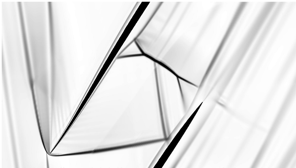
Figure 5.27: Numerical Schlieren picture of the cascade: shockwave pattern in the blade passage
