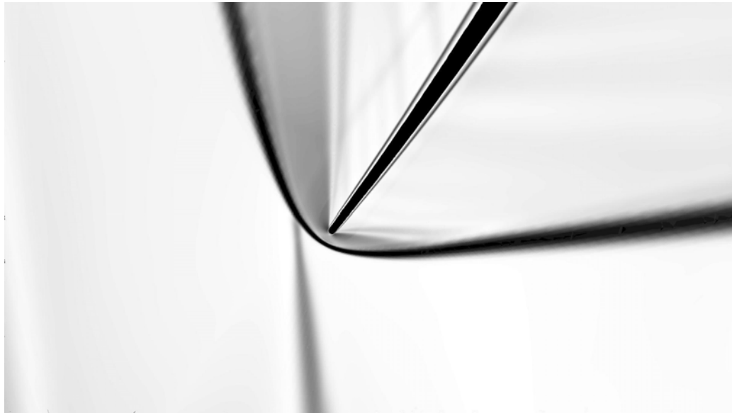
Figure 5.26: Numerical Schlieren picture of the leading edge: close-up of the bow shock and the precompression shock
