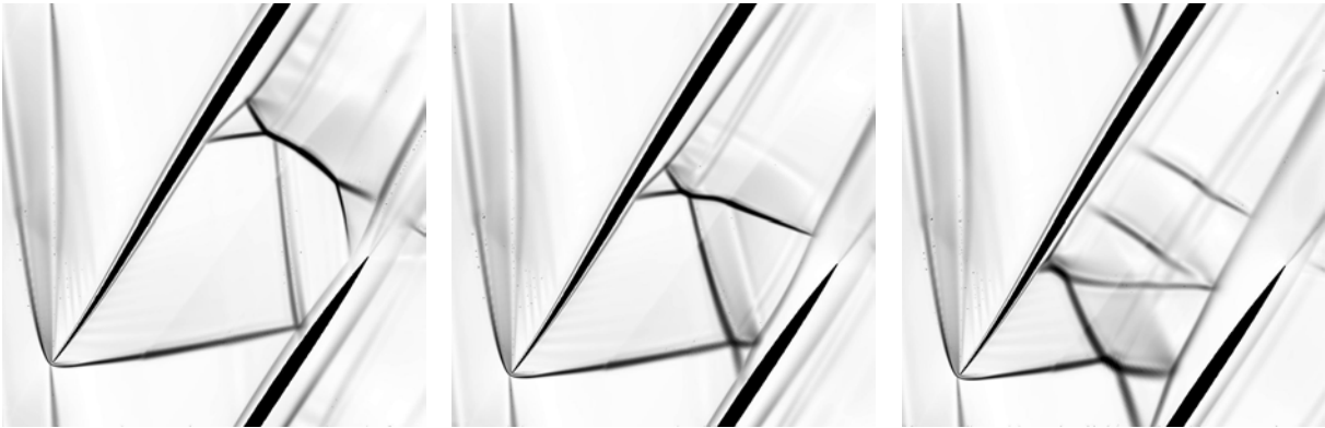
Figure 6.24: Numerical Schlieren pictures of the cascade flow field at different static pressure ratios for \sigma = 1.5294
