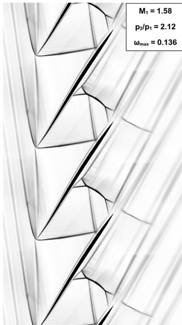
Figure 6.20: Example of the shock wave pattern at maximum total-pressure loss point
