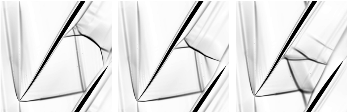
Figure 6.25: Numerical Schlieren pictures of the cascade flow field at different static pressure ratios for \sigma = 1.60
