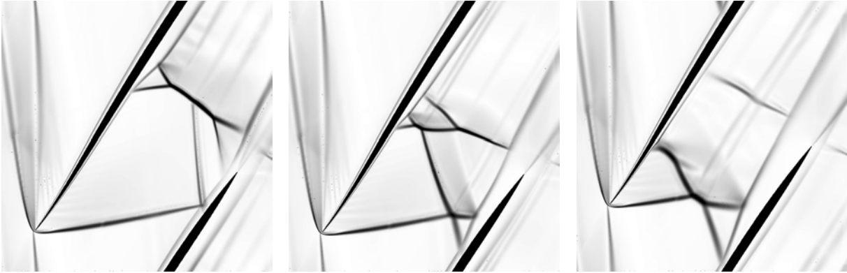
Figure 6.23: Numerical Schlieren pictures of the cascade flow field at different static pressure ratios for \sigma = 1.47
