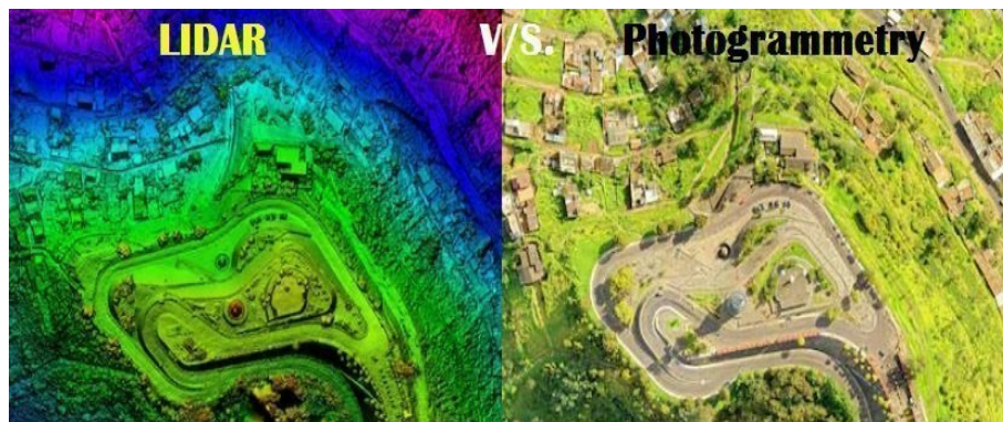
Figure 3: Comparing Photogrammetry with LiDAR for the same scene
