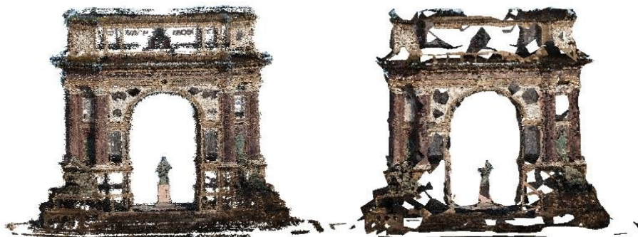
Figure 7: Arco Valentino PC: left) original PC; and right) MPEG G-PCC decoded PC. Original texture used for recoloring.
