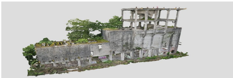
Figure 2: Example of point clouds acquisition by photogrammetry
