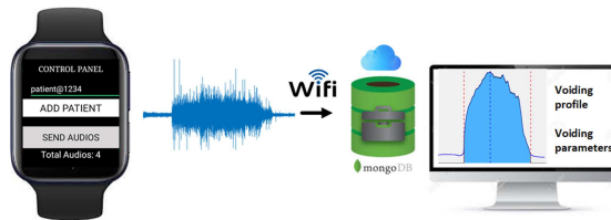
Figure 2.3: Architecture of the platform: The UroSound App facilitates the wireless transmission of audio files to a distant web server through WiFi for signal processing and feature extraction. The securely stored audio files are managed in a MongoDB database.
