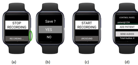
Figure 2.4: User interface of the UroSound App for Wear OS: (a) Initiating the UroSound App and automatically commencing audio recording is achieved by pressing the lower-right button highlighted in green. (b) Upon tapping 'STOP RECORDING' on the screen, a dialog prompts the user to save or discard the recorded audio. (c) Commencing a new recording is facilitated by tapping 'START RECORDING' on the screen. (d) The concealed control menu, not visible to the users, is utilized for patient registration and the transmission of audio files to a remote database.
