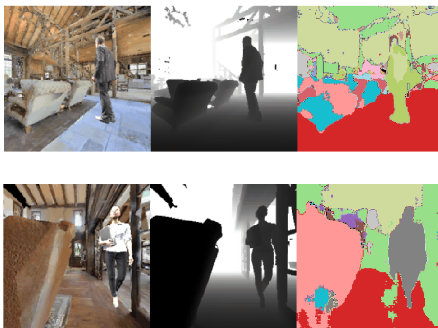
Figure 7.1: Output provided by the not fine-tuned RedNet (top) and the output provided by the fine-tuned RedNet(bottom). As we can notice the not fine-tuned RedNet is not able to recognize correctly the class person by assigning multiple classes to it.
